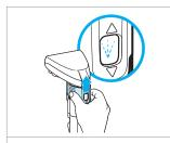
7. Slide tool lever up to ensure tool is in SPRAY mode.
