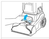
1. Lift the accessory hose door on top of foot on the front of the machine. The door flips toward the machine to open.
