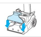
7. To reinstall the nozzle, align the ribs on the ends of the nozzle to the machine, then lower the nozzle into place.
