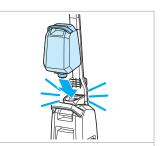
**6.** Push clean tank down. Ensure it is seated securely on the base
